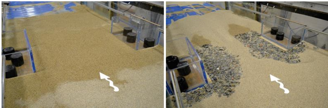
Figure 71. Photos. Comparison of run 6 as-built riprap installation (left) and at equilibrium scour (right).
