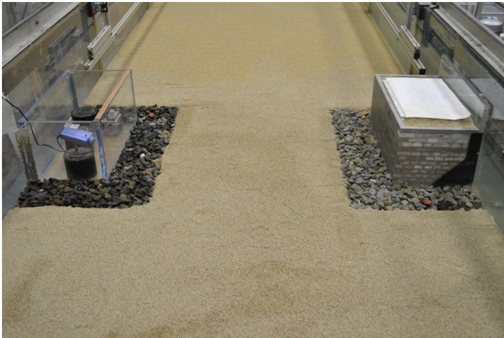
Figure 57. Photo. Vertical-wall abutment models installed in the test section.
