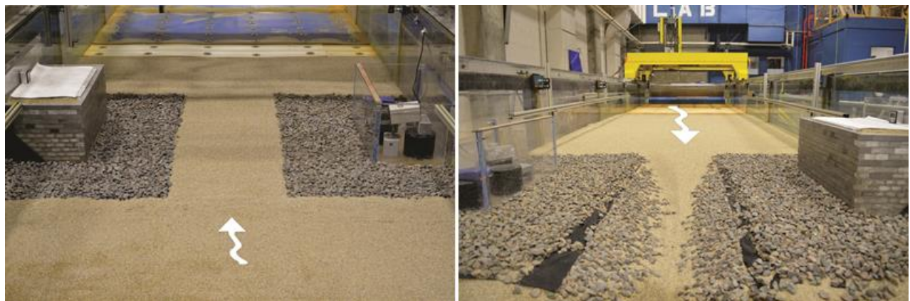
Figure 61. Photos. Comparison of run 1 as-built riprap installation (left) and at equilibrium scour (right).
