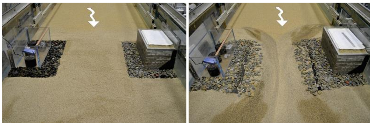
Figure 69. Photos. Comparison of run 5 as-built riprap installation (left) and at equilibrium scour (right).
